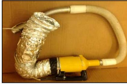
Vac set up for blow filling cavity on the gable end of my bungalow surprisingly quickly.
